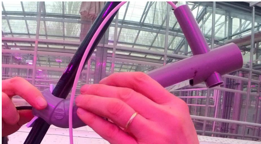
Figure 11. Assembly of the sensor enclosure on the pole.
