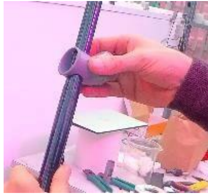
Figure 12. Mounting the sensor support on the mast
