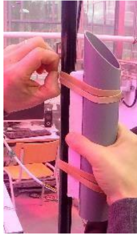
Figure 10. Attachment of the main enclosure to the mast
